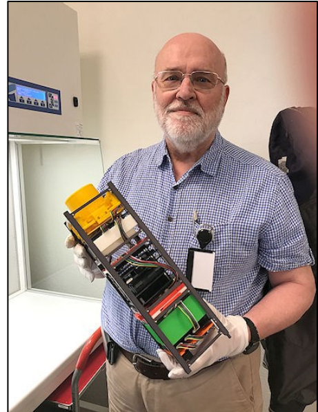
Figure 37 First iteration of the Engineering model w/ 3D-printed experiments held by the team leader.
