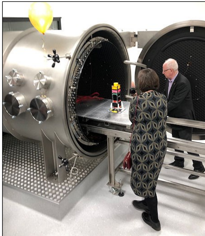
Figure 45 The MIST EM with 3D-printed experiments in the KTH vacuum test chamber at its inauguration, spring 2019.
