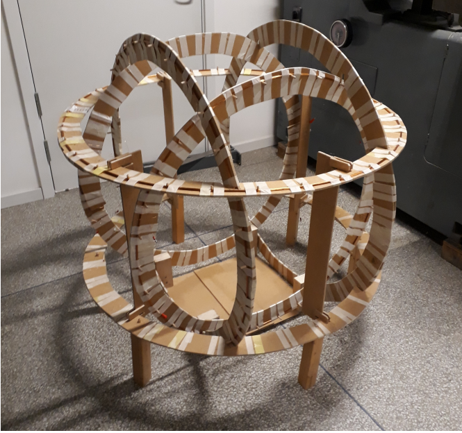
Fig. 7. The three-axis Helmholtz coil assembly, the smallest coil pair defines the X-axis, the intermediate Y, and the largest, horizontal pair is Z.
