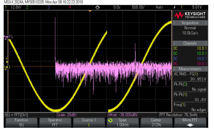
Fig. 11. Sine wave produced using rotatingfield.ino on the circuit (yellow), and the frequency distribution calculated by the FFT function on an oscilloscope (pink).
