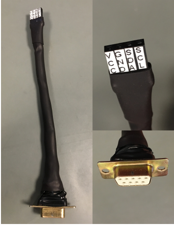
Fig. 5. The 9-pin female D-sub attached to four wires with pin headers for the four inputs of the male D-sub on the AntS simulator
